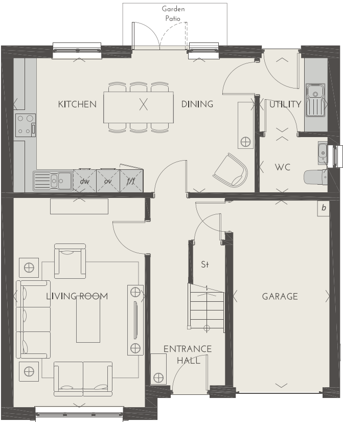
Legend: b - boiler f/f - tall integrated fridge freezer ov - tall integrated oven and microwave dw - integrated dishwasher St - store
